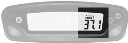
Fig 6 Adjustable trip distance function
